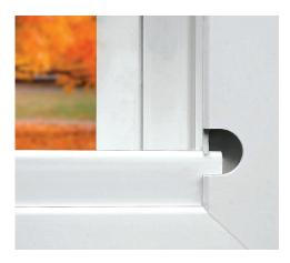
The sill dam wall is mortised into the jamb adding strength and lowering the possibility of leaks that may occur at corner seals.
