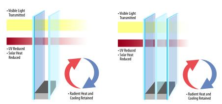
In climates where heating and cooling are the primary concern, HeatSeal® Glass products are designed to take advantage of free solar heat, resulting in higher inside glass temperature. Passive solar and thermal insulation reduce the draft sensation caused by cold glass surfaces, providing windows that reduce heating costs.
