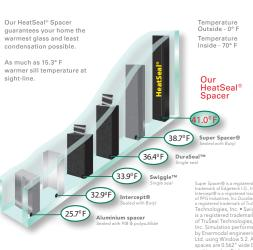
Examples of Condensation: A good quality spacer can significantly reduce condensation in comfortable humidity levels. Water and ice forming can lead to mold arowth.
