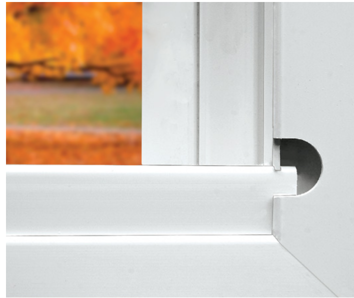
The sill dam wall is mortised into the jamb adding strength and lowering the possibility of leaks that may occur at corner seals.
